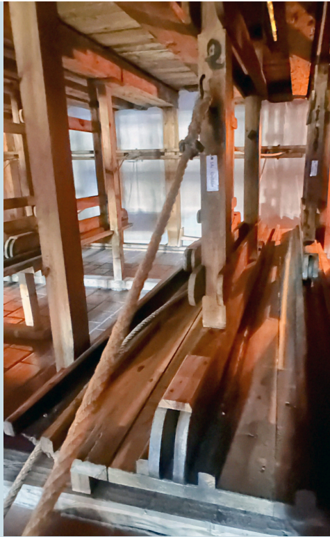
A detail of the Chariot-and-Pole scene changes system housed below the stage of the Baroque Theater. Photo courtesy of Kiara Pipino.
