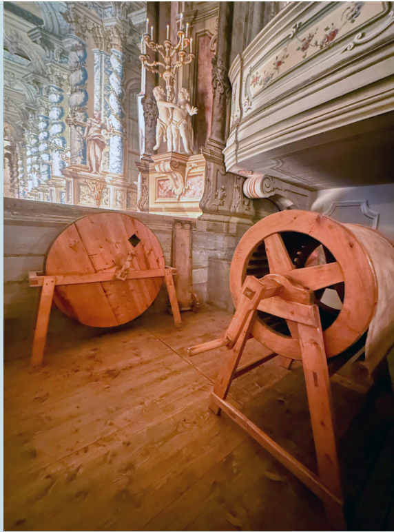
Examples of the machinery used for special effects. At the back, close to the stage, a round spinning wooden wheel would generate rain sounds. Next to it, a vertical wooden plank with smaller dented wheels would be used to simulate thunder sounds. Finally, the wooden spinning barrel topped with fabric would be used to generate wind sounds. Photo courtesy of Kiara Pipino.
